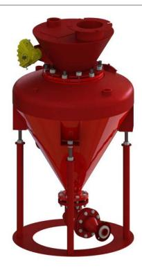
The cone section of the pressure vessel is fabricated using a press break in order to maintain the same metal thickness throughout the cone section, and all pressure vessel designs include leg supports that are adjustable. The adjustable legs allow vital internal components to be easily accessed for inspection or maintenance.
