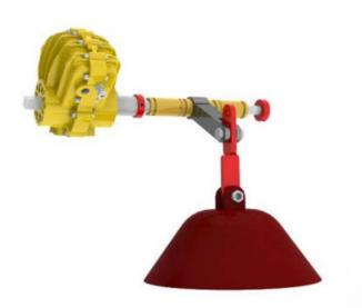
The Dense Flow Cone Valve features robust components designed for use with abrasive materials, and in one application a cone valve lasted 18 years in a system conveying sand at 20,000 #/Hr. 24/7/365 before needing replacement. Its design creates a stronger seal as the pressure within the conveying system increases, allowing it to hold pressure at 125 psi and beyond.
