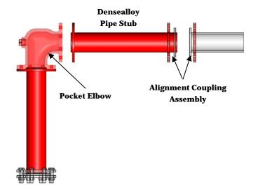
The Densealloy Pipe Stub was designed as an alternative to replacing an entire length of pipe. Our engineers found that on most pneumatic pipelines the most wear occurred within the first two feet after an elbow or bend. Also, because the Pipe Stub is only two feet in overall length it is replaced must easier than entire length of pipe.
