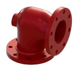
The pocket traps material which then acts as a barrier for any remaining material moving through the elbow. Material in a pocket elbow will have less contact with the actual elbow body and material moves slower in a pocket elbow versus a traditional sweep bend. Less contact and lower material velocity translates into an elbow that will last up to **10 times longer** than a traditional sweep bend.
