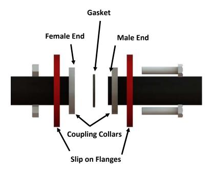
Coupling collars are welded on the two ends of pipe that are being joined, one end creates a male connection and the other a female connection. Two 150# B.C. slip on flanges compress a gasket between the two coupling collars to insure an air tight seal up to 125psi.
