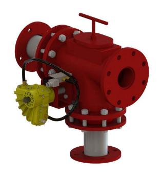
The diverter valve features a pocket design where the initial incoming material is trapped at the valves deflection point, and then acts as a barrier from the remaining material being conveyed.
