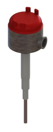
The control board is protected by a dust tight aluminum housing, and is easily accessed through a threaded cap. The probe itself is stainless steel, and probe function can be tested while the unit is installed.
